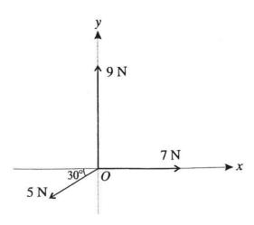
Three horizontal forces act at the point O. One force has magnitude 7 N and acts along the positive x-axis. The second force has magnitude 9 N and acts along the positive y-axis. The third force has magnitude 5 N and acts at an angle of  $30^{\circ}$  below the negative x-axis (see diagram).
