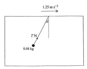
An object of mass 0.08 kg is attached to one end of a light inextensible string. The other end of the string is attached to the underside of the roof inside a furniture van. The van is moving horizontally with constant acceleration 1.25 m s<sup>-2</sup>. The string makes a constant angle  $\alpha$  with the downward vertical and the tension in the string is T N (see diagram).
