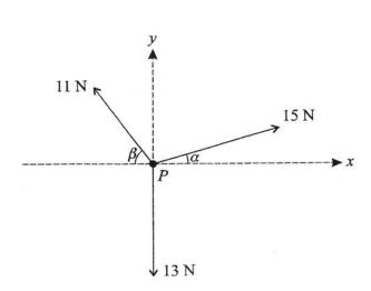
Three horizontal forces of magnitudes 15 N, 11 N and 13 N act on a particle P in the directions shown in the diagram. The angles  $\alpha$  and  $\beta$  are such that  $\sin \alpha = 0.28$ ,  $\cos \alpha = 0.96$ ,  $\sin \beta = 0.8$  and  $\cos \beta = 0.6$ .
